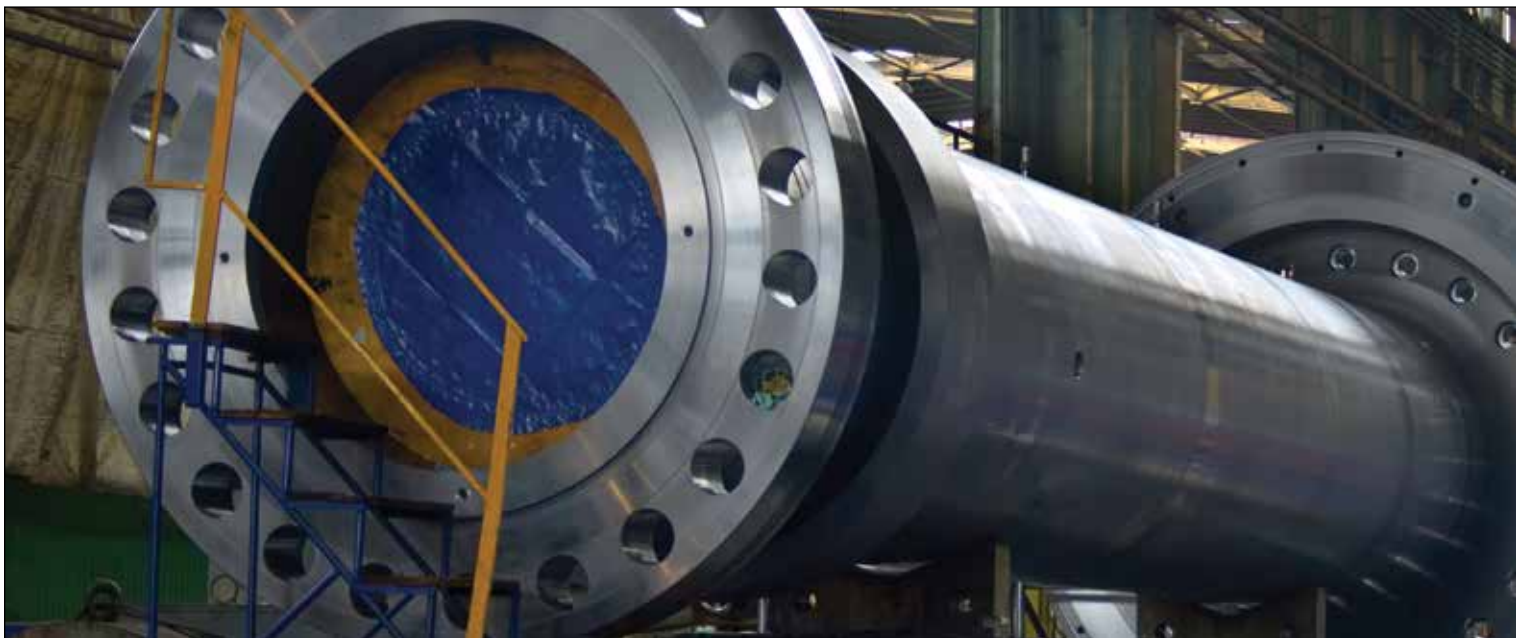
Nook/Thomson machine screw jacks are used in large material transfer applications.
