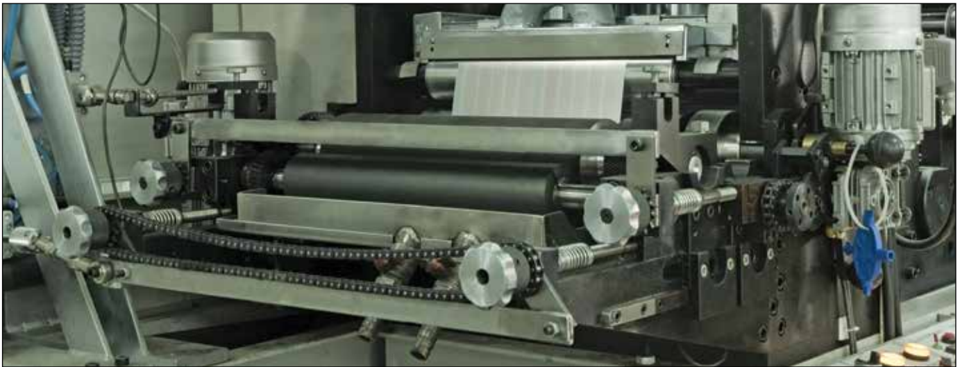
This printing press application utilizes two upright translating ball screw jacks to set the proper gauge on the feed rollers.
