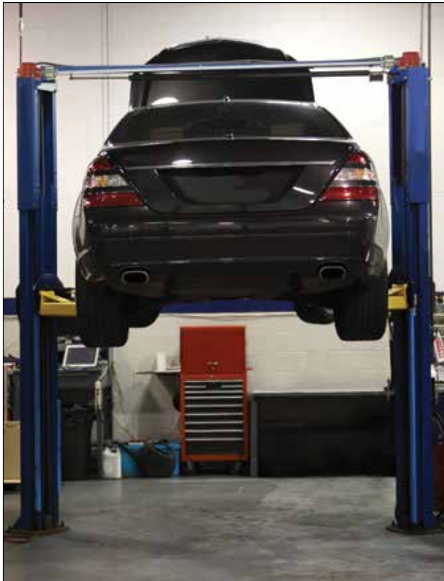
In this automobile lift, the linear motion is provided by two inverted rotating ball screw jacks.
