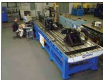
High Load Modular Test System 40,000 lb load - 100" CC
