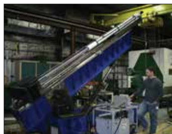
Convertible Test System 20,000 lb load - 100" CC
