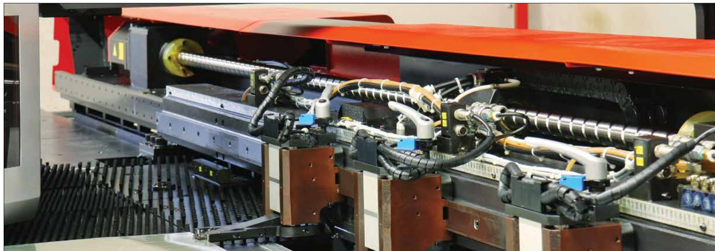
CNC welding machine using precision ground ball screw
