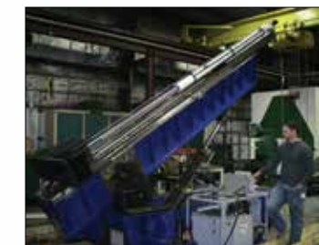
Convertible Test System 20,000 lb load - 100° CC
