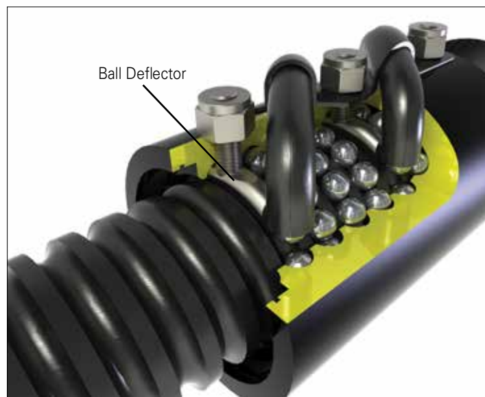
Ball nut with ball deflectors
